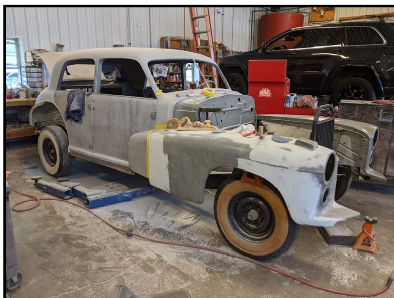
Body stripped and primed – panel fitment underway
