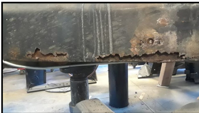
Rust in the bottom of the right rear door
