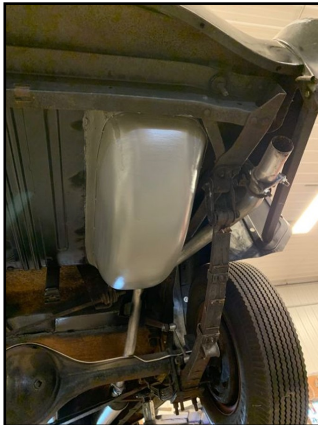
New spare tire well installed
