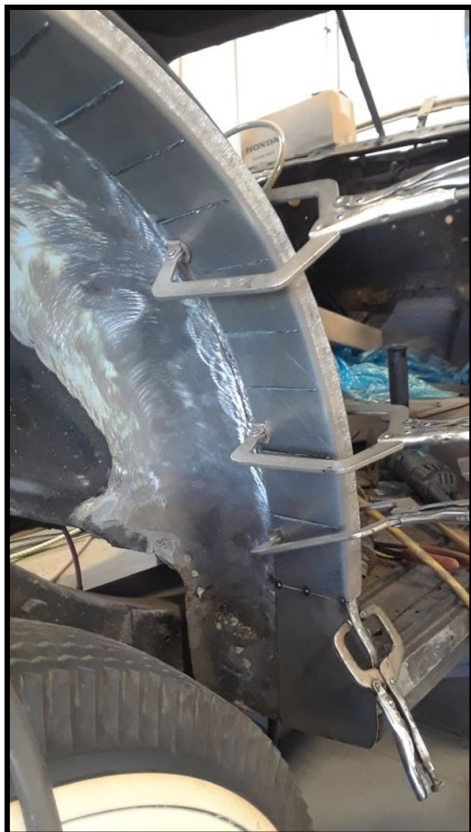
Rust repair in the right rear wheel arch
